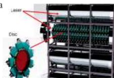
Figure 1: Artist's rendering of a single disk laser module and its replication to form a complete high-energy laser system. Multiple such lasers are combined to provide redundancy and scalable output for a fusion power plant.
